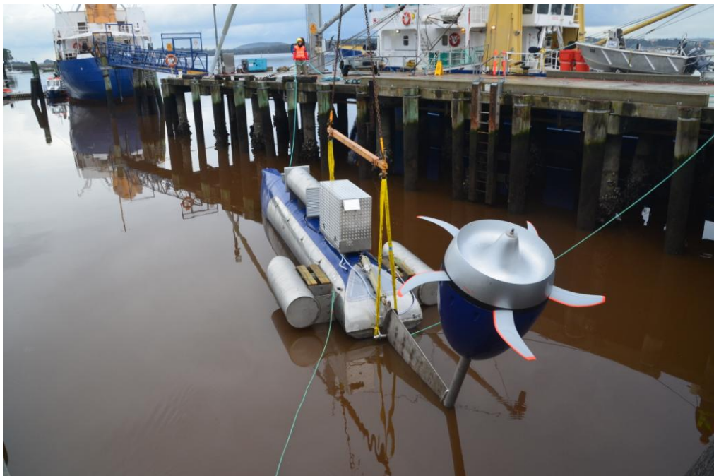
MAKO tidal turbine in an upright position before being towed to the deployment site at which point the fin holding the turbine was lowered to a vertical position to hold the turbine horizontally in the tidal flow to spin the five carbon fibre blades and produce electricity from the onboard generator.
