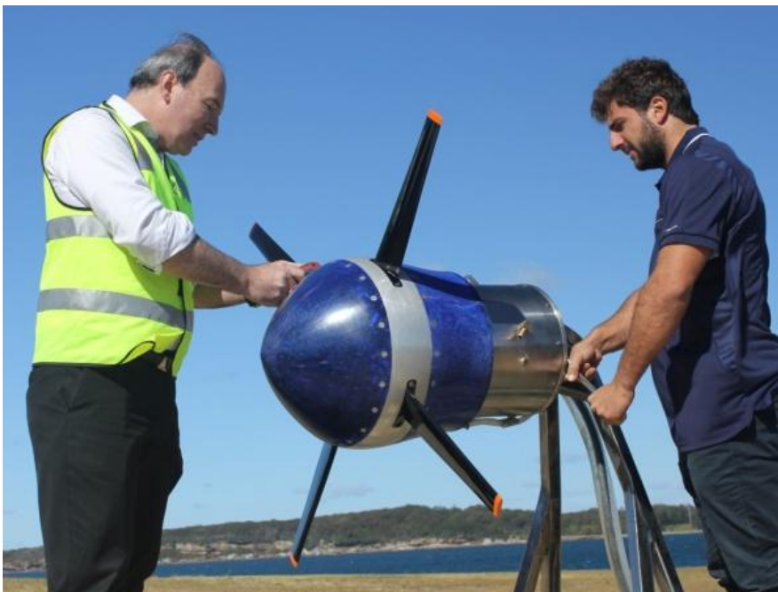
Photo: MAKO Tidal Turbines is pioneering an initial range of small-scale tidal turbines designed to minimise shipping, installation and maintenance costs, particularly in remote locations.
